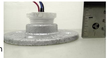
About ¾" of clearance above the female threads (measured from the top of the PVC sensor threads) is required to install this sensor (please also account for any adapter you will be using). The below adapter can be purchased at any plumbing store.
